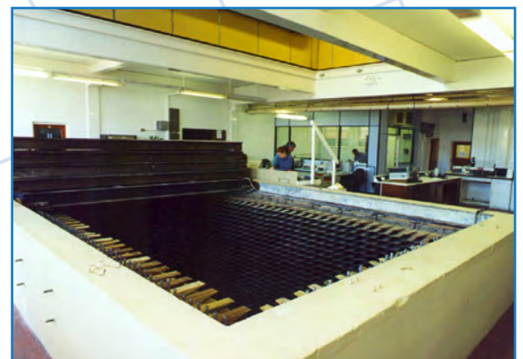
The in-house Acoustic Test Tank hosts a computer-controlled transducer test and calibration facility
